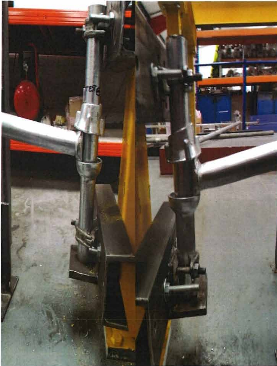
Cyclic Ledger Tube Test 6 - Before & After
